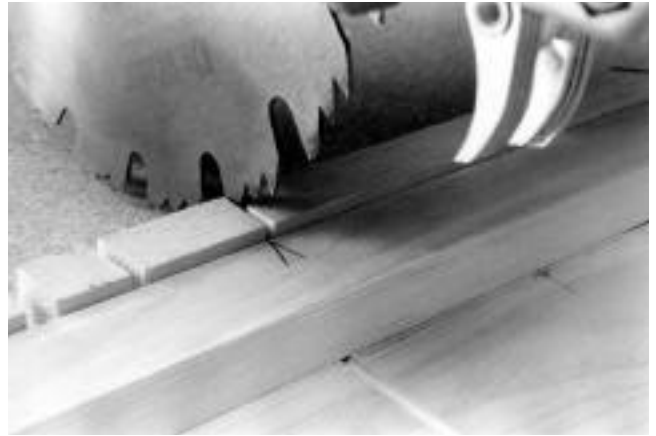
Fig. 2-1: the fence as an alignment tool for cross cutting
